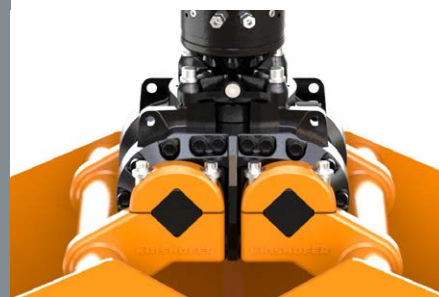
Loosen 4 bolts on each side
